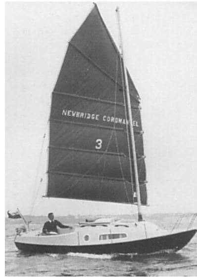
Fig. 2 Junk-rigged 21 foot Coromandel by Newbridge Boats: sailhandling without tears.
