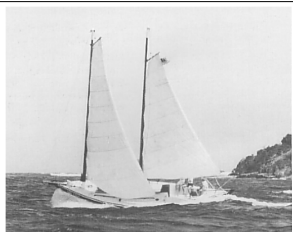
Fig. 1. Choppy conditions, but the crew of this unstayed cowhorn schooner Sea Legs can control each sail from the cockpit.
