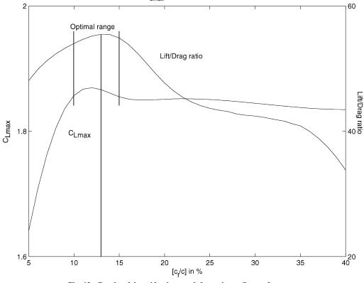
Fig. 13 Results of the grid point search for optimum flap performance.
