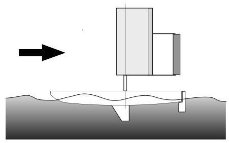
Fig. 16 Conventional configuration with the tail behind the wing.
