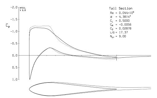
Fig. 11 Pressure distribution of the final tail section at a Reynolds number of 44,000 and a lift coefficient of 0.5.
