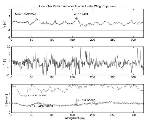
Fig. 2 Sailing path errors, cross-track error (top), heading error (center), and boat and wind velocities (bottom).
