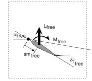
Fig. 25 Close-up view of the forces and moments on the free-floating canard.
