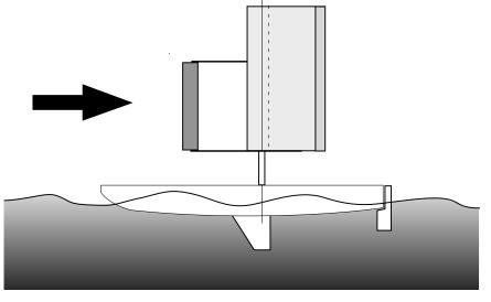
Fig. 18 Canard configuration, tail ahead of the main wing.
