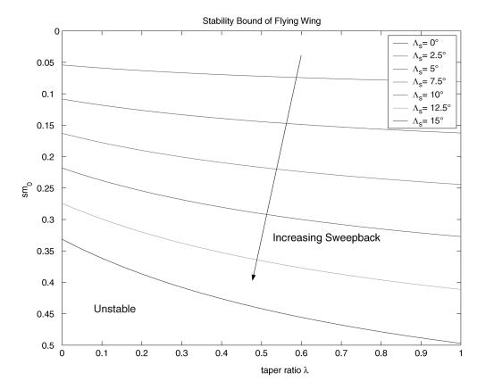
Fig. 22 Stability bound plot for flying wing configuration with a quarter-chord sweep angle  $\Lambda_s$ , taper ratio  $\lambda$ , and mast pivot offset point  $sm_0$ .
