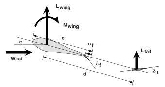
Fig. 17 Forces and moments on the conventional configuration.
