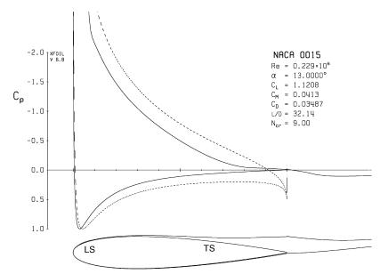
Fig. 8 XFOIL results for NACA 0015 airfoil at Reynolds number of 229,000 and C<sub>L</sub> of 1.12.
