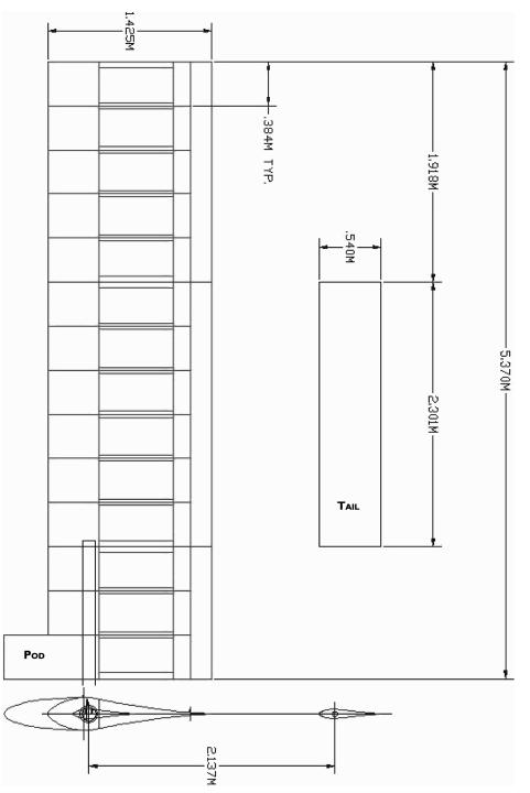
Fig. 5 Engineering layout of the wingsail.
