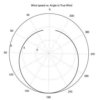
Fig. 7 Polar plot of the true wind speed vs the angle to the true wind for a Reynolds number of 229,000.
