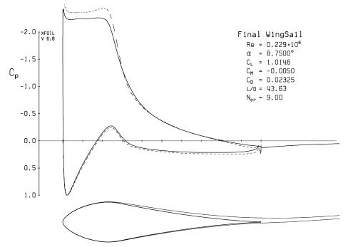
Fig. 10 Final wingsail airfoil section and pressure distribution, Reynolds number of 229,000, and a lift coefficient of 1.0.
