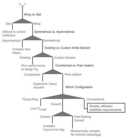
Fig. 4 Design evolution of the wingsail propulsion system.
