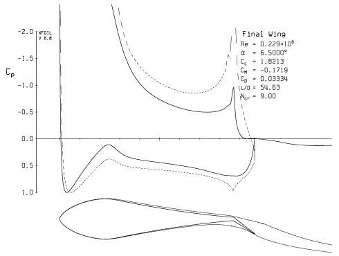
Fig. 12 Pressure distribution of main wingsail section with flap deployed, *Re* of 229,000 and a C<sub>L</sub> of 1.8.
