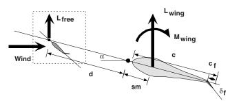
Fig. 24 Forces and moments on the free-floating canard configuration.
