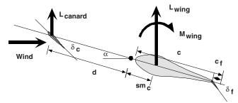
Fig. 19 Forces and moments on the canard configuration. Distances *d* and *sm* are measured positive aft of the pivot point.
