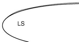
Fig. 9 Close-up view of the laminar separation bubble on NACA 0015 airfoil at Reynolds number of 229,000.
