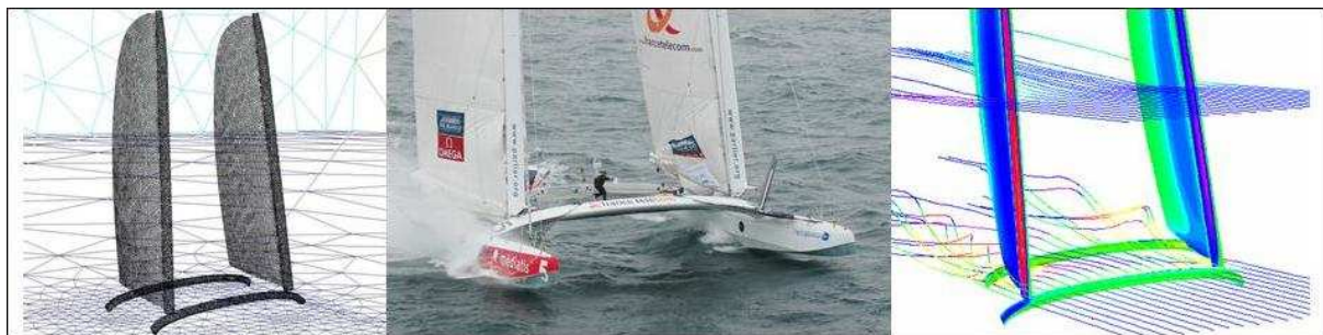
Figure 1: Hydraplaneur twin rig with two mainsails and no jib. (Left) an example of three dimensional mesh for RANS simulations, (center) Hydraplaneur at sea, (right) an example of RANS flow solution
