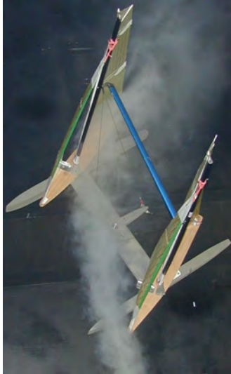
Figure 13: deviation of the air stream between the windward and leeward rigs.
