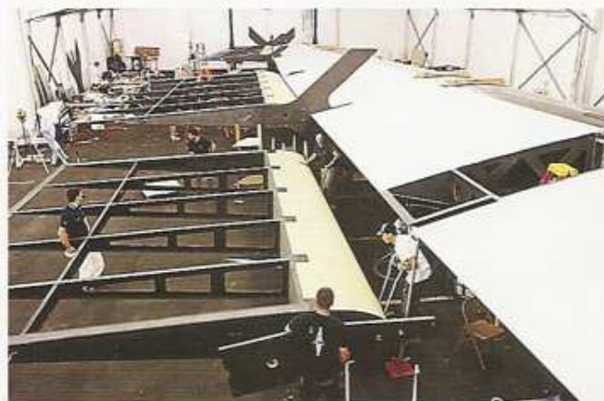
Left: prior to skinning the sections a flap forest was raised in the tent in San Diego, transport issues requiring everything to be assembled in situ next to the yacht. The breathtaking precision and finish quality of even the largest components (above) – in six months, remember
