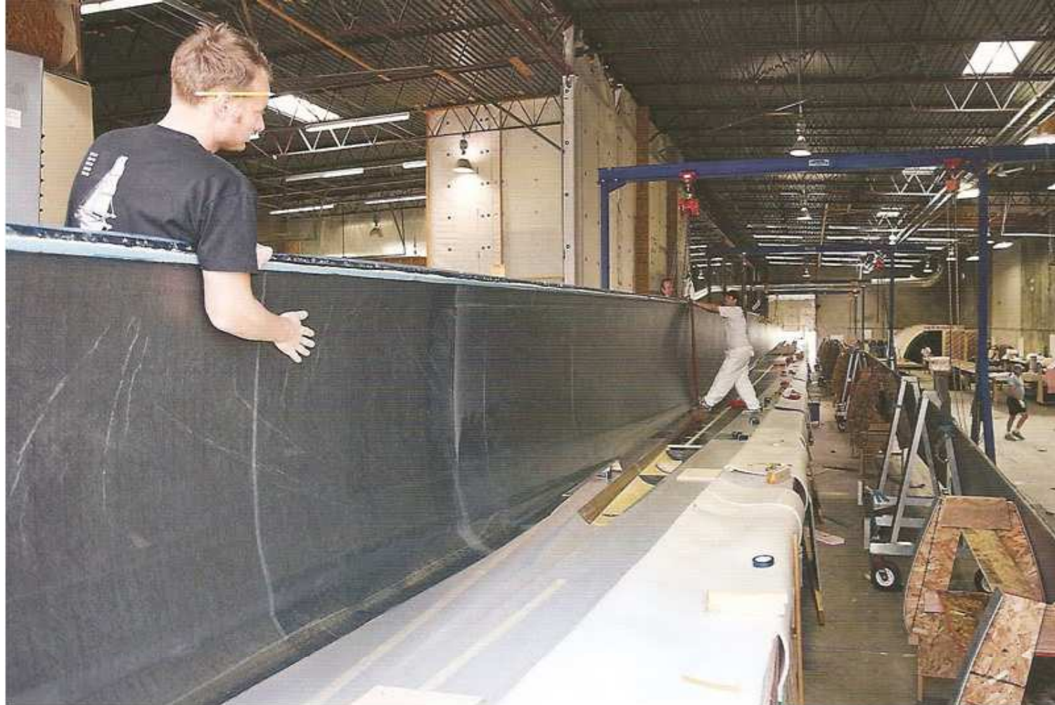
The starboard top half side panel of the main spar is offered up to the nose cone tool beneath it. The correct alignment of such long and slender components was a constant challenge and lasers were in use non-stop in the effort to ensure everything stayed in a straight line
