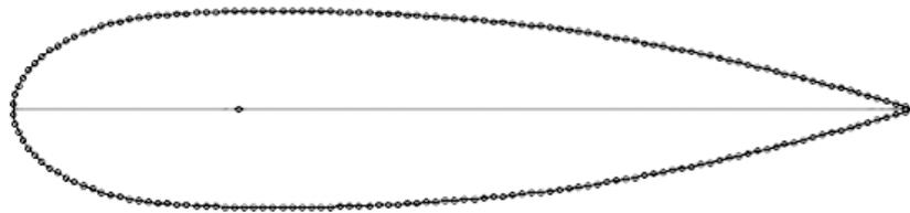
Figure 3.3: Aerofoil section of main wing (trailing edge not deflected)
