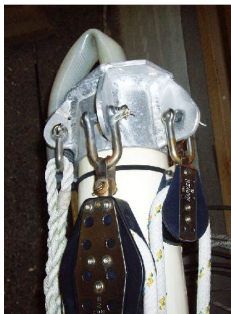
Johanna's masthead (aluminium) From left to right: Mastlift, halyard - and halyard; I use 2 blocks. Note plastic hose on top which covers the lantern wire. For size reference; the lines are 10mm.
