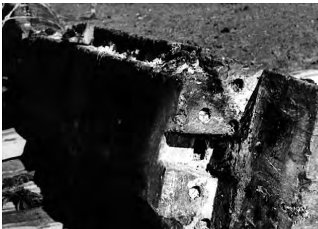
Figure 77. Photograph of keel scarf at the time of excavation showing the baosongkong .
