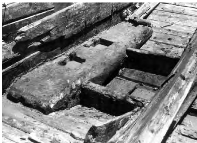
Figure 80. The main mast step at time of excavation, note longitudinal braces.
