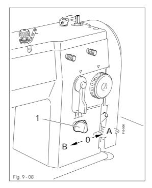
• Set the required stitch position with stitch position adjustment lever 1.
