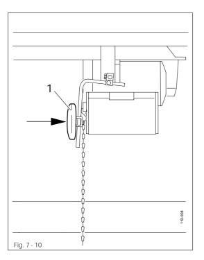
• Depending on the type of assembly, by pressing knee lever 1 either the presser foot is raised or the zig-zag stitch width altered.
