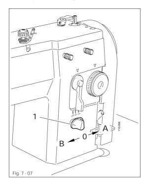
• To set the required stitch position adjust the stitch position adjustment lever 1.
