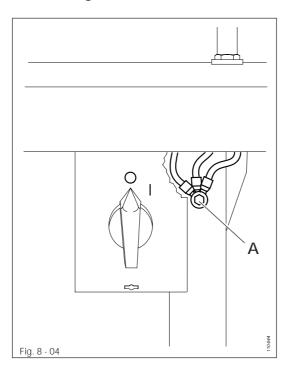
• Screw the earth cables from the sewing head, main switch and motor to earth point **A**.
