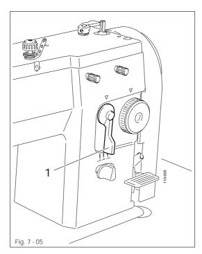
• To adjust the width of the zig-zag stitch operate the zig-zag stitch lever 1.
