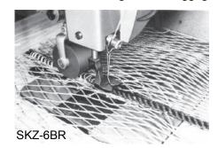
\*Suit for repairing fishing net Puller performs exact stitching, by fixing flexible materials, thus suitable for sewing and repairing vinyl made fishing net, etc.
