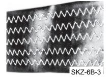
\*Suit for sewing elatic and stretching materials Three steps zig zag stitching suitable for sewing elastic and stretching materials on foundation. (Sewing type 308)
